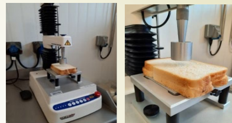
Figura 4.4. a) Texture Analyzer (TA.XT Plus, Stable Micro System, UK); b) sonda 35 mm
