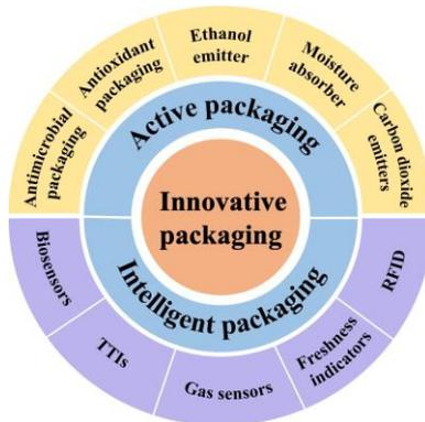
**Figure 4.2.** Classification of innovative food packaging systems. (TTIs: time-temperature indicators; RFID: radiofrequency identification)
