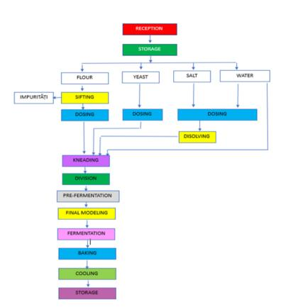
Figure 5.2. Technological flow of bakery process
