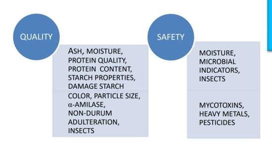
**Figure 6.4**. Semolina quality parameters and their influence on pasta quality and safety (after Turnbull, 2001)
