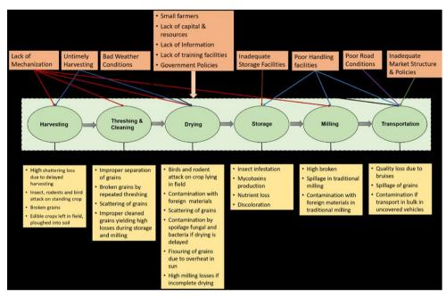
Figure 4.13. The factors and types of losses during the supply chain of cereal crops in developing countries. Taken from Kumar and Kalita, 2017 (https://www.mdpi.com/2304-8158/6/1/8) Copyright 2020 Creative Common Attribution License
