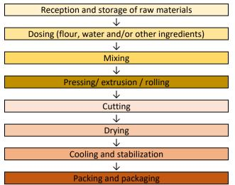
Figure 6.1. General technological diagram of pasta production (after Klinger 2010)
