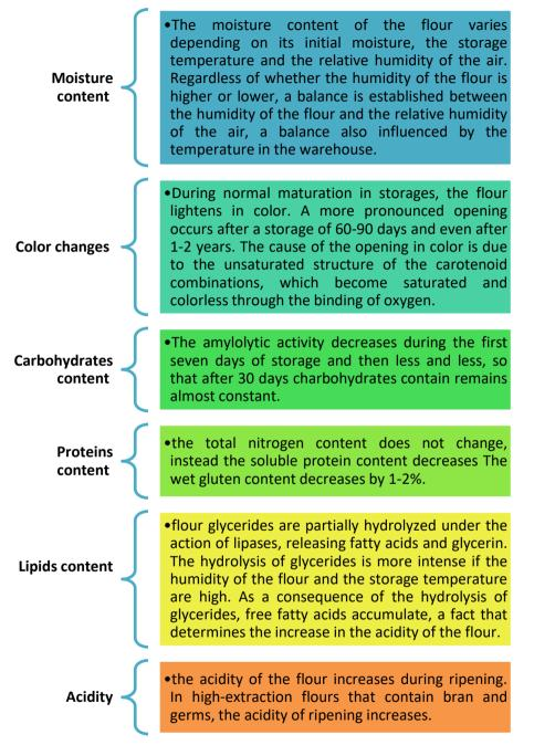
**Figure 3.3.** Processes that take place during flour storage on which the quality of bakery products and FW depends
