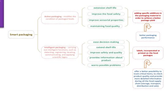
Figure 4.3. The characteristics and the roles of smart packaging
